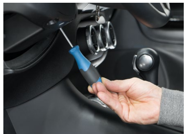
The locking device for the ignition key can be overridden using a screwdriver
